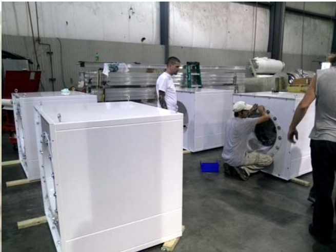
Fan Modules in final assembly at Seasons 4
