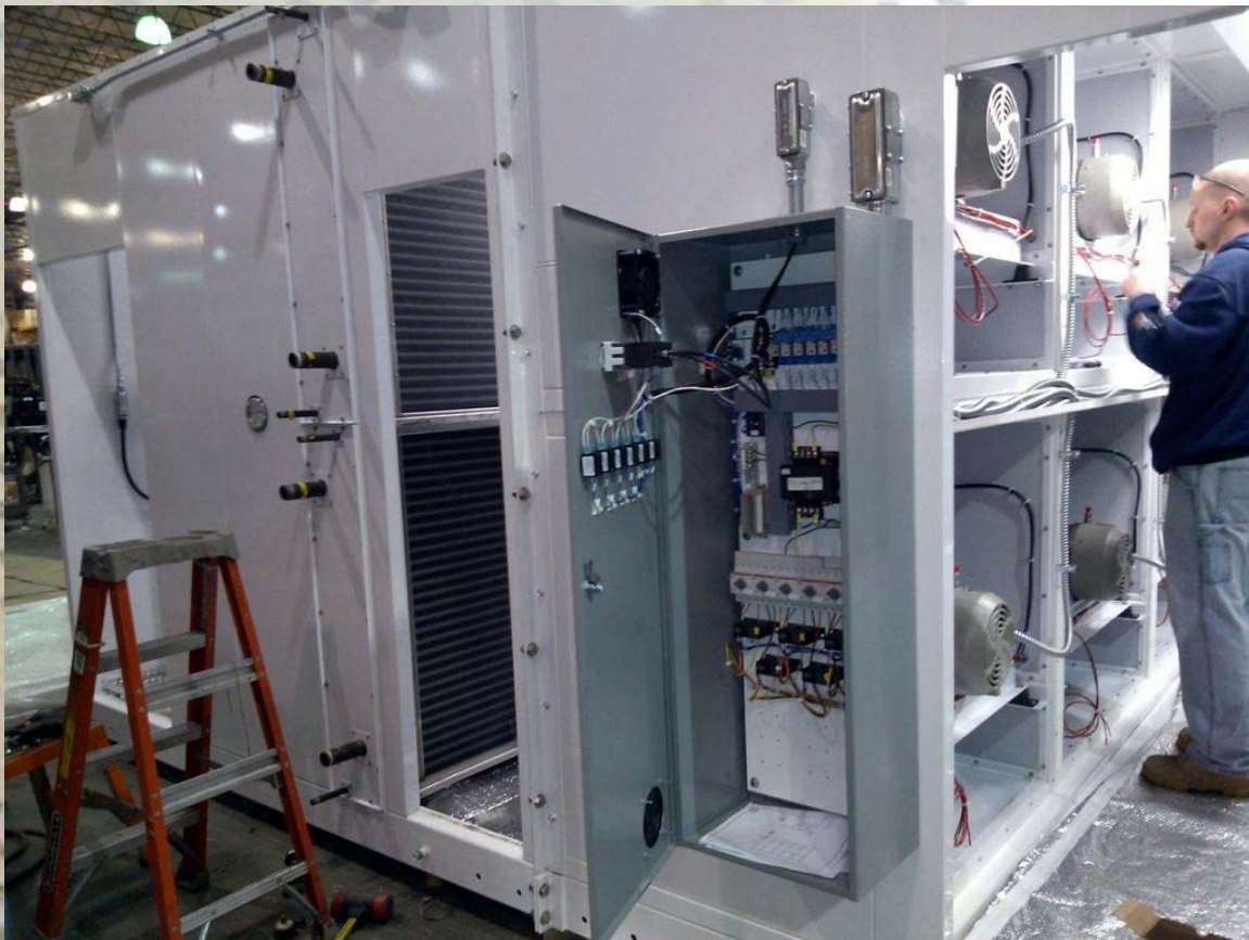
50,000 CFM CLEANROOM RECIRCULATION AIR HANDLER
