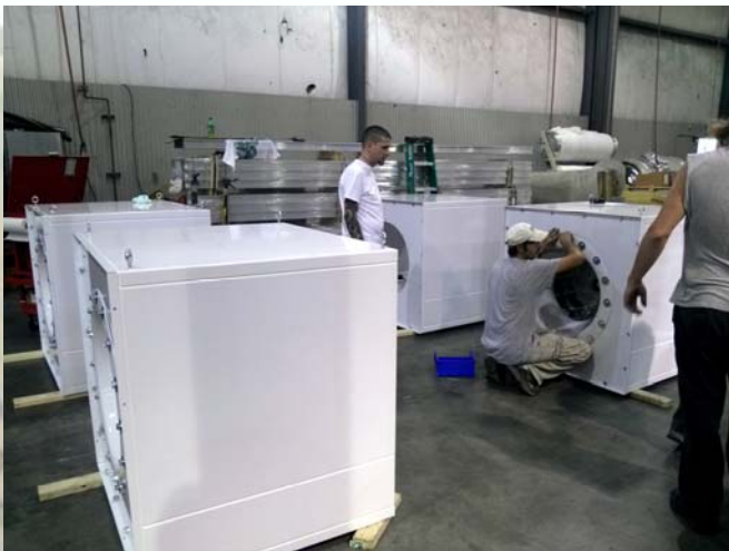
Fan Modules in final assembly at Seasons 4
