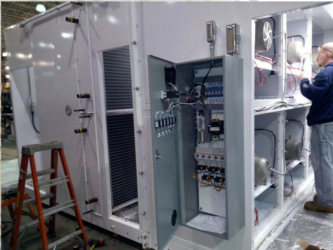
50,000 CFM CLEANROOM RECIRCULATION AIR HANDLER
