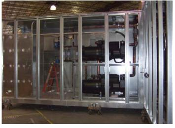
The new unit will have two (2) evaporative condensing sections with two (2) 80 ton Copeland screw compressors per section. The units are designed to match the existing curb without any field supplied refrigeration piping and fully charged with R-134A refrigerant at the factory.
