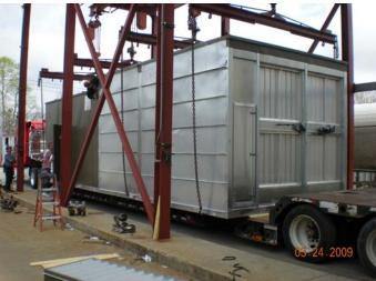
Kynar painted aluminum exterior panels, lights in all accessible sections are additional features. The sections are bolted and wired together for testing and then split into sections and shipped to the jobsite..
