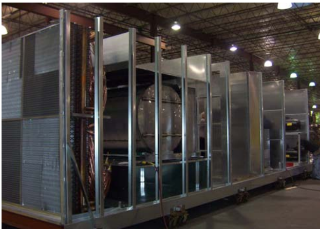
High turndown natural gas power burner with stainless steel drum and tube heat exchanger
