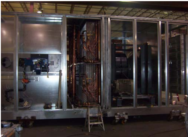
Evaporative condenser, airfoil plenum blower with 60 HP premium efficiency motor
