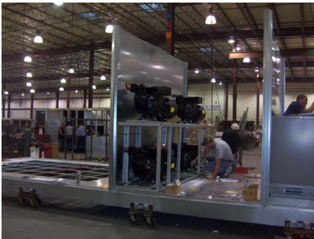
(4) Copeland screw compressors mounted in a walk in service vestibule with aluminum diamond tread plate floor.
