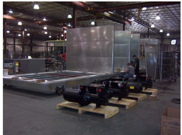
(4) Copeland screw compressors mounted in a walk in service vestibule with aluminum diamond tread plate floor.
