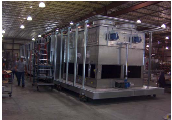
Evaporative condenser, airfoil plenum blower with 60 HP premium efficiency motor
