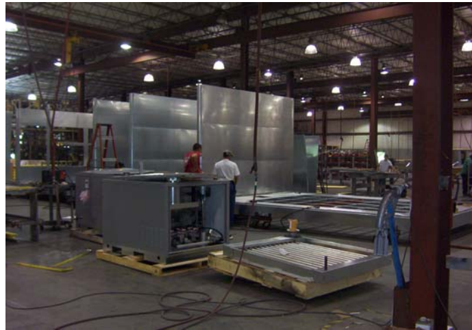
900 LB/HR natural gas-fired self-contained humidifier with modulating controls.
