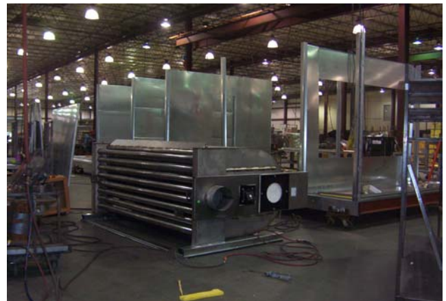
High turndown natural gas power burner with stainless steel drum and tube heat exchanger
