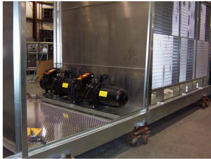
Air cooled condensing section, service vestibule with tread plate floor and screw compressors.
