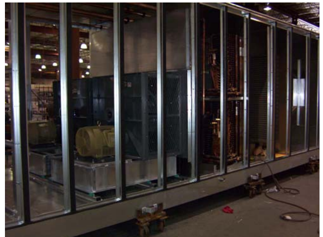
Air cooled condensing section, service vestibule with tread plate floor and screw compressors.
